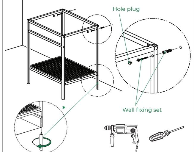
\* - If you have a plinth along the wall that interferes with the installation of the frame, then the rear legs can be unscrewed..
