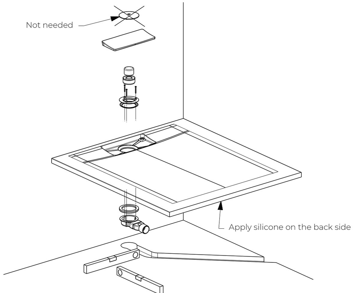
1. Place the shower tray in position on the floor (ensuring surface is level) and mark the perimeter, drain and trap.
