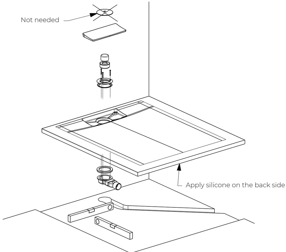
1. Place the shower tray in position on the floor (ensuring surface is level) and mark the perimeter, drain and trap.
